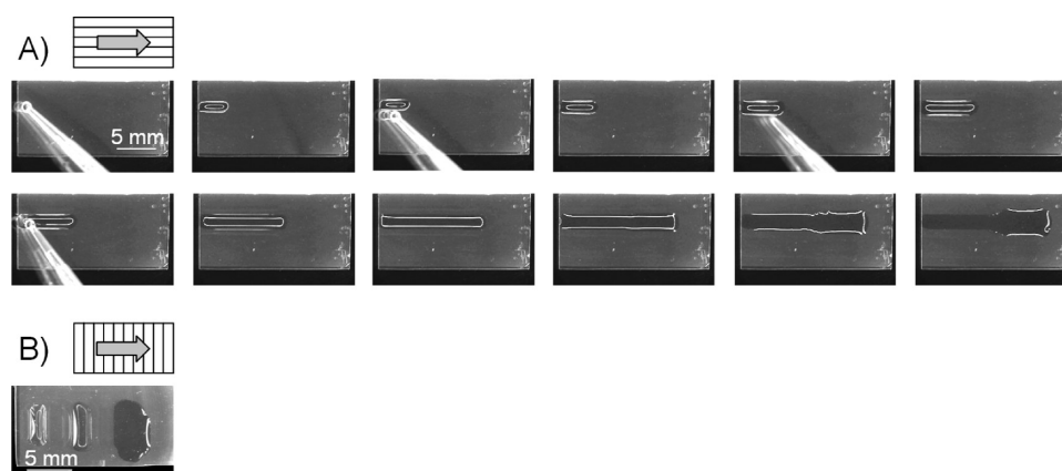
Figure 7. Illustration of the spreading of water droplets on surfaces with periodic grooves and a superimposed polymer brush wettability gradient. The cartoons illustrate the orientation of the grooves and the direction of the gradient (arrow pointing from the high CA to the low CA side. (A) First row: Series of snapshots showing how three droplets ( 1.5 \mu\text{L} each) were dispensed on the high CA side of the gradient. Second row: dispensing of a fourth droplet results in spreading over the whole length of the gradient and dewetting on the high CA side. (B) Photograph of drop spreading on a surface having the gradient direction oriented perpendicularly to the hot embossed grooves.
